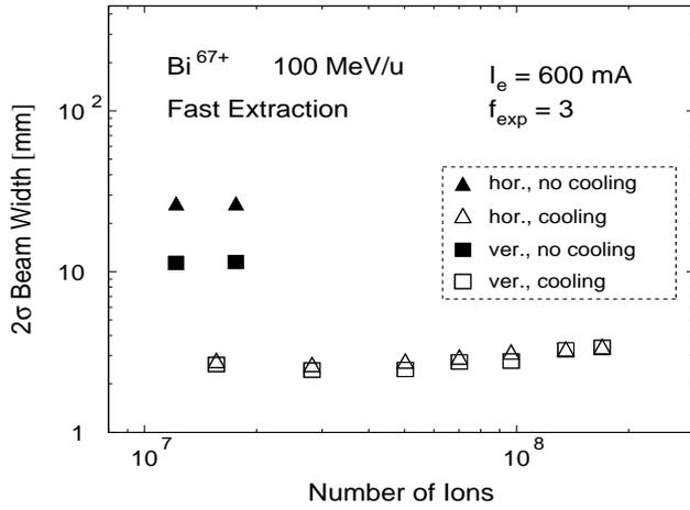
Figure 3: Horizontal and vertical beam size of the fast extracted ion beam ( $\text{Bi}^{67+}$  at 100 MeV/u) without and with cooling at the injection energy.
