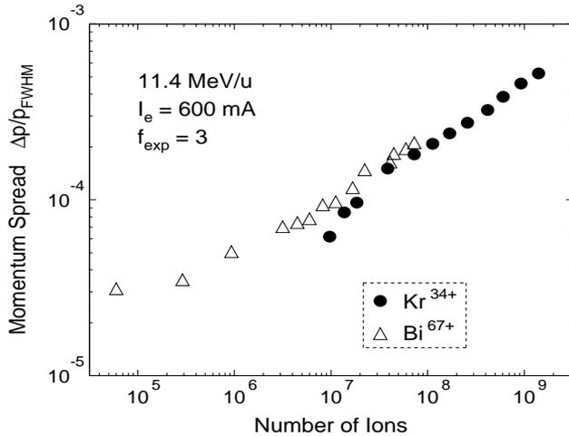
Figure 4: Momentum spread of the accumulated cooled ion beam at the injection energy 11.4 MeV/u. The electron beam of 600 mA was expanded by a factor of 3.
