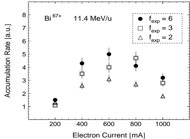
Figure 2: Accumulation rate for a  $\text{Bi}^{67+}$  beam as a function of the electron current for three expansion factors.
