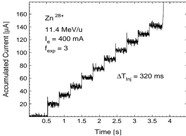
Figure 1: Ion current growth during cooler assisted beam accumulation. The  $\text{Zn}^{28+}$  beam was cooled at the injection energy 11.4 MeV/u with a 400 mA electron beam expanded by a factor of 3.
