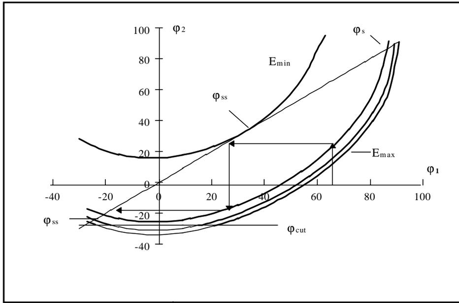
Fig. 2. Initial phase of electron emitted from electrode 2 in dependence on initial phase of electron from electrode 1 at different values of electric field gradient.
