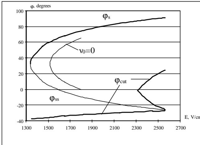
Fig. 3. Phase lines against electric field gradient.
