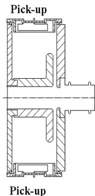
Fig. 1. Schematic view of the beam phase monitor.
