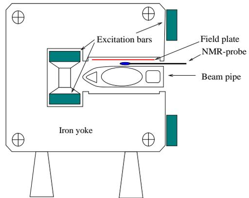
Figure 1: Cross section of the instrumented LEP dipole. The NMR probe is mounted in top of the chamber and below the field plate, which is glued on the pole surface.
