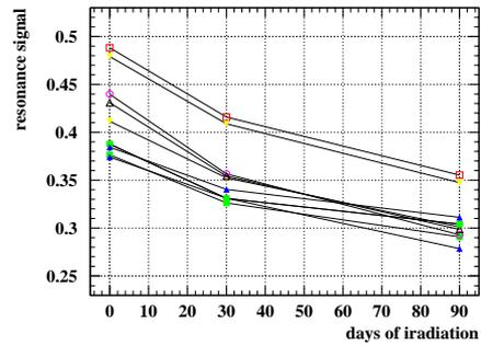
Figure 4: Variations of the NMR probe resonance signal. Top: Increase of the resonance signal of two probes with increasing field. Bottom: Decrease of the resonance signal with time of operation (irradiation time).
