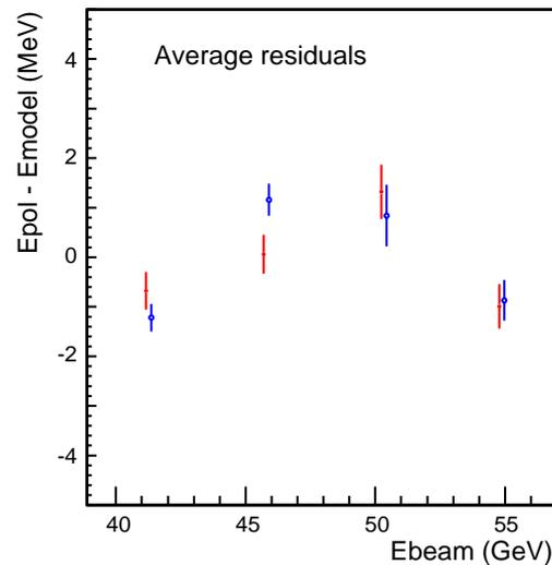
Figure 6: Residual beam energy variations for different beam energies comparing the resonant depolarization calibrations and the beam energy estimated using NMR probes.
