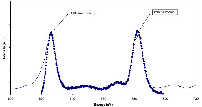
Figure 3: 11<sup>th</sup> and 12<sup>th</sup> harmonic at 23.5 mm gap with Landau cavities tuned in giving energy spread 0.22 %. Dots - measured, solid line - simulated.
