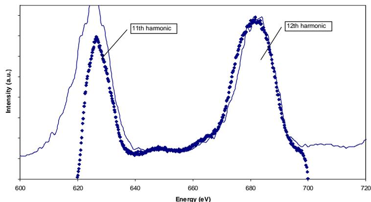
Figure 2: 11<sup>th</sup> and 12<sup>th</sup> harmonic at 23.5 mm gap. Landau cavities tuned out and energy spread 0.4 %. Dots - measured, solid line - simulated.
