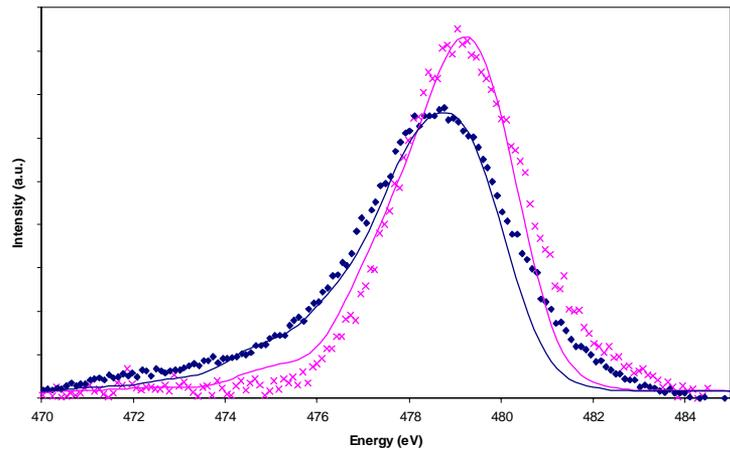
Figure 1: 8<sup>th</sup> harmonic at 24 mm gap. Coupled beam (wide peak) and uncoupled beam (narrow peak), Dots/crosses - measured, solid line - simulated.
