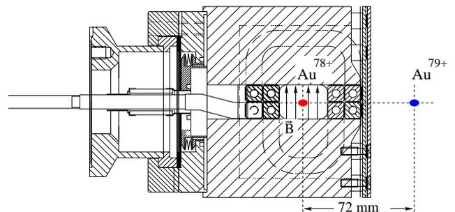
Figure 3: Side view of the movable magnetic septum. Also shown are the primary  $\text{Au}^{79+}$  and the down-charged  $\text{Au}^{78+}$  beam which are separated about 72 mm at the septum.
