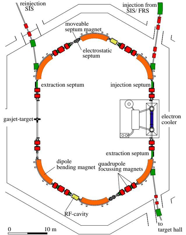
Figure 1: Storage ring ESR with its main components.
