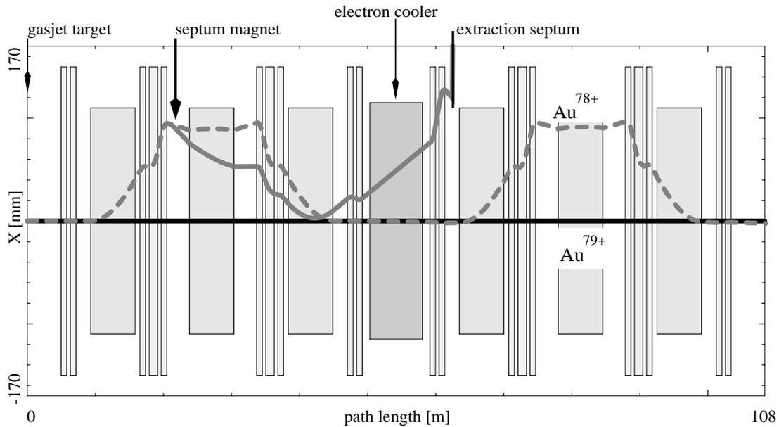
Figure 2: Horizontal separation of the orbits of a primary and secondary Gold-beam along one revolution in the storage ring. The extracted secondary beam is deflected into the extraction septum by a small kick in the north bend of the ESR.
