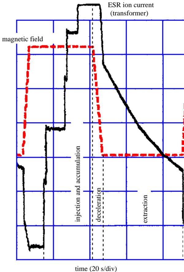
Figure 4: Typical ESR cycle for experiments with decelerated beams and charge exchange extraction.
