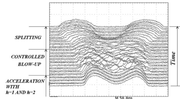
Figure 2 : Splitting and blow-up at the end of acceleration in the PSB ( $3 \times 10^{12}$  protons).
