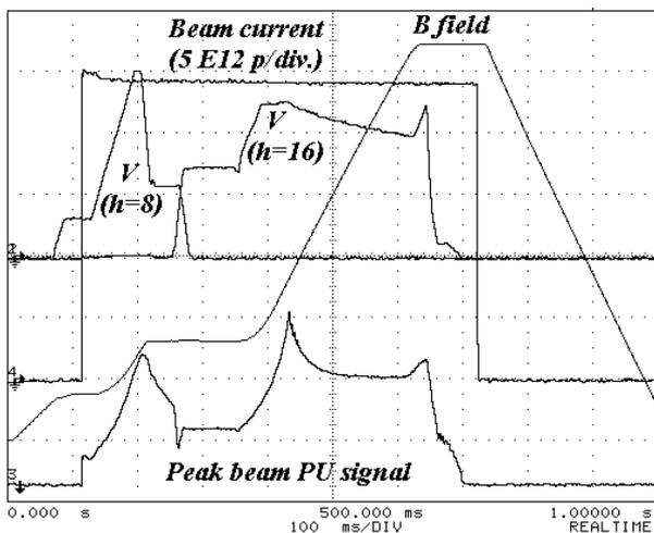
Figure 3: Full PS acceleration cycle for SPS.
