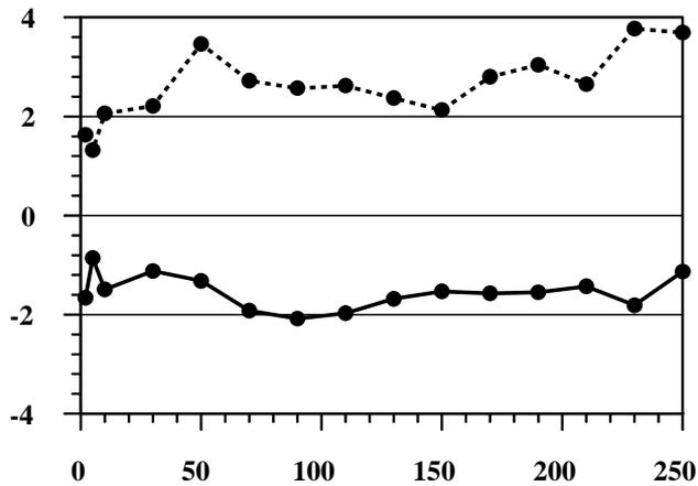
Figure 2: Measured horizontal beam positions [mm] at monitors P1 (solid) and P2 (dotted) as a function of energy step
