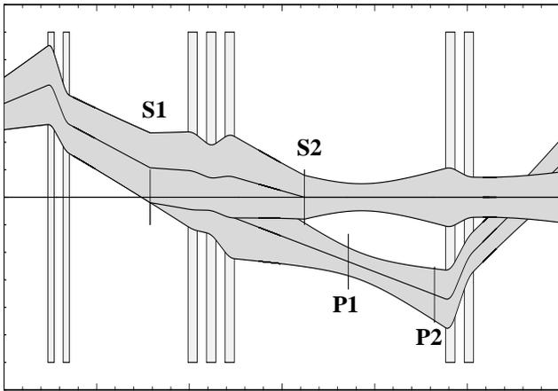
Figure 1: Principle of position correction using MIRKO: position measured at P1 and P2, back transformation to the start, and correction with steerers S1 and S2
