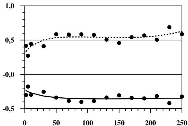
Figure 3: Calculated steerer settings [mrad] (dots) and fitted polynomes for S1 (solid line) and S2 (dotted line)
