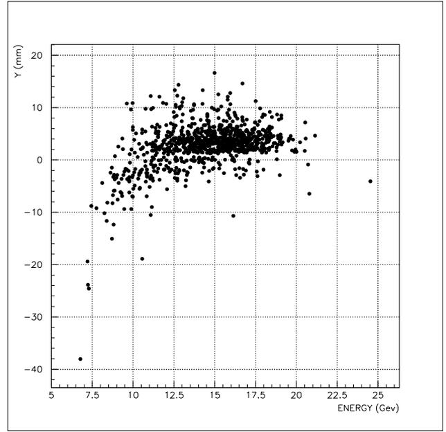
Figure 2: Dependence of electron vertical displacement at electron tagger plane on electron energy
