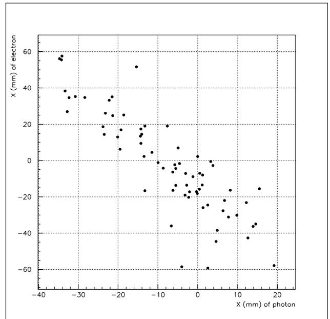
Figure 3: Scatter plot of the horizontal displacement of the bremsstrahlung photons at PD vs the horizontal displacement of the secondary electrons at ET
