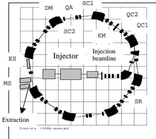
Figure 2: General layout of the accelerator complex.
