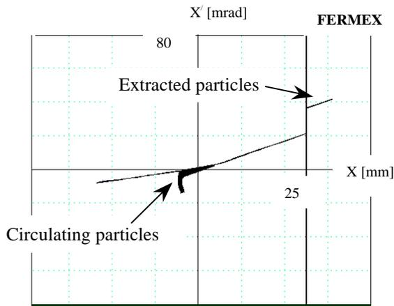
Figure 5: Transverse phase-plane of the extracted beam with the momentum spread ( $-0.001$ ).
