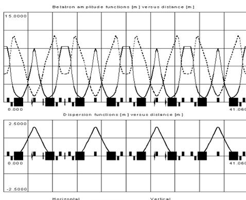
Figure 3: Twiss parameters of the focusing structure.
