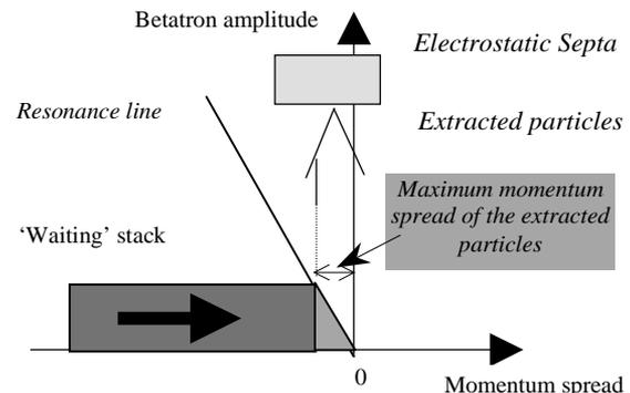
Figure 1: Steinbach diagram of the amplitude-momentum extraction technique.
