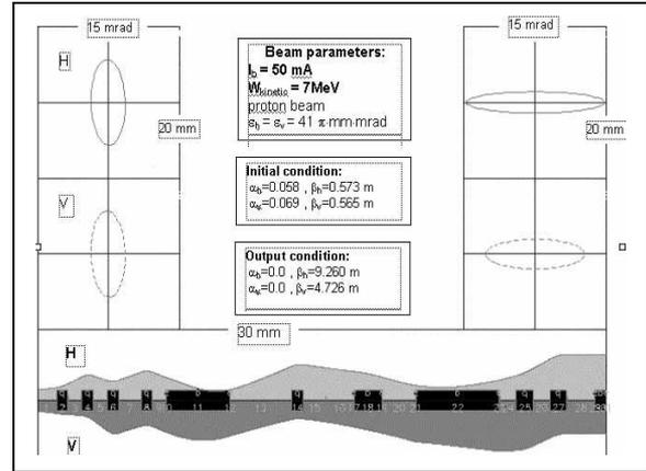
Figure 6: Beam envelope along the injection beamline.
