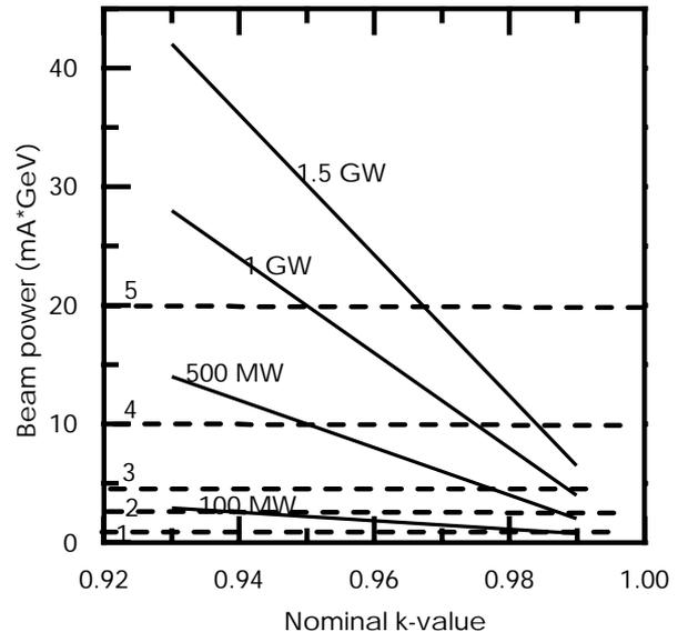
Figure 1: Required power of proton beam versus reactor multiplying coefficient. Dashed line means: 1- PSI - 1.8 mA, 0.59 GeV, 2- PSI - 5.0 mA, 3 - DC - 2.5 mA, 1 GeV/nucleon., 4- DC - 5.0 mA, 5 - DC -10.0 mA.
