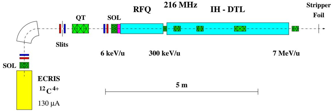
Figure 1: Schematic drawing of the designed carbon injector LINAC.
