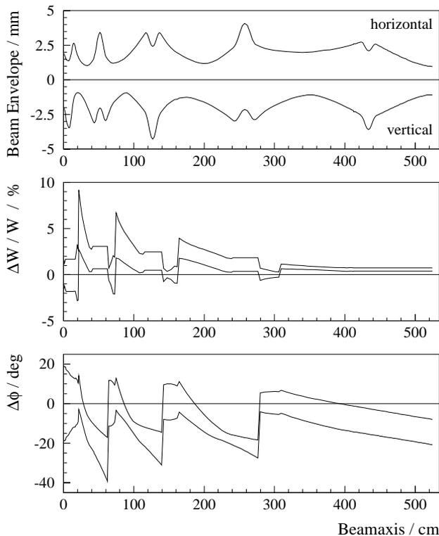
Figure 2: 98 % beam envelopes within the IH-DTL, including the intertank beam-matching section and up to the stripper foil (compare to Fig. 1). The IH cavity begins at an axial coordinate of about 17 cm and ends at about 414 cm. For longitudinal beam matching two drift tubes integrated in the RFQ cavity are included in the simulations.
