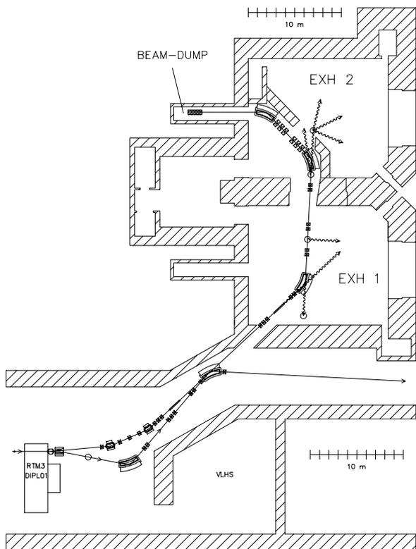
Figure 2: Transport system for the X1 experiments.
