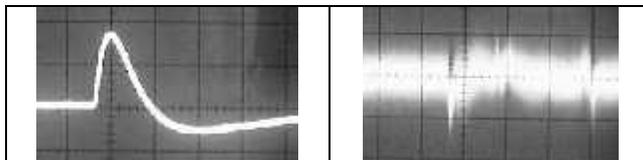
Figure 3: Rf-monitor signals. *Left*: 2mm displacement of the pulsed beam. *Right*: Centred beam (0.06mm/div.).
