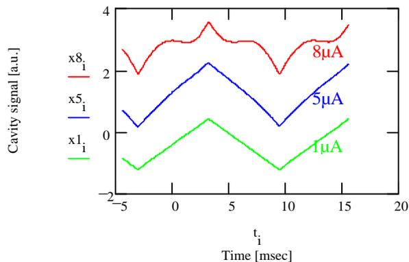
Figure 6: Horizontal beam motion in turn 90 at different cw beam currents.
