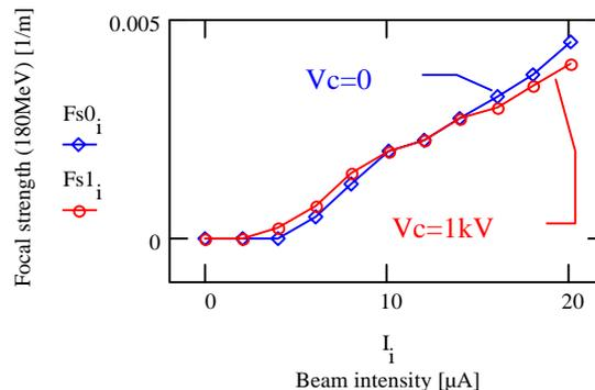
Figure 7: Additional focusing by ion-trapping.
