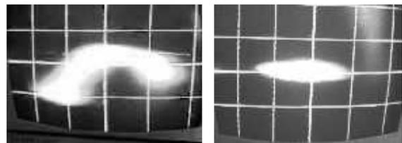
Figure 1: Longitudinal phase space at the entrance of the injector linac (above) and at 3.5MeV with standard (right) and with harmonic prebuncher (15% resp. 50% total transmission). Screen cal.: 2°/div. hor. and 4keV/div. vert.
