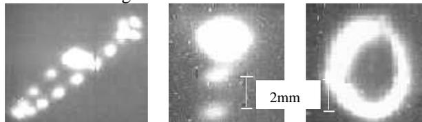
Figure 4: Beam spots from synchrotron radiation at the end of the accelerator axes. In RTM2 (left) the last 15 turns and in RTM3 the last 2 turns are displaced. On the right the different beams in RTM3 are displaced one by one to form a circle.
