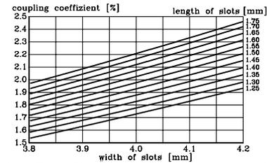
Figure 11: Coupling coefficient versus slot width for some slot lengths. Geometry is as in figure 10 at 12 GHz.
