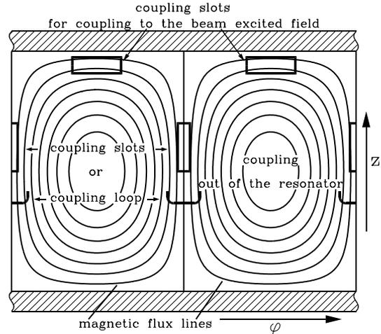
Figure 1: Principal mode of operation of the resonant BPM.
