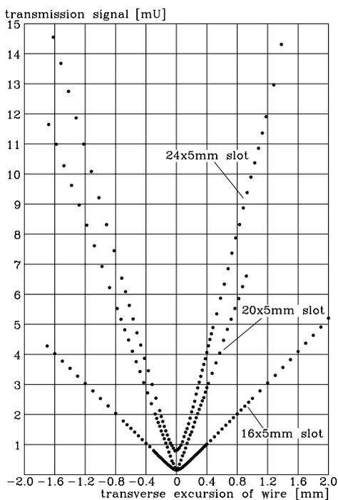
Figure 3: Measured transmission coefficient versus the wire shift for three different slot lengths for prototype A.
