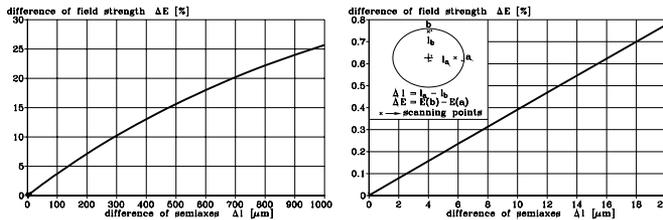
Figure 8: Relative difference of the field strength versus the ellipticity of the beam tube with a centered beam, taken at constant distance from the center of the ellipse.
