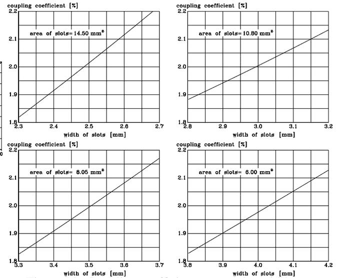
Figure 10: Coupling coefficient versus slot width at constant area. Dimension of TEM-line is  $5 \times 15$  mm, of X-band rectangular waveguide  $22.86 \times 10.16$  mm at 12 GHz.
