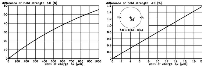
Figure 7: Relative difference of field strength versus the shift of the beam in an exact round beam tube.
