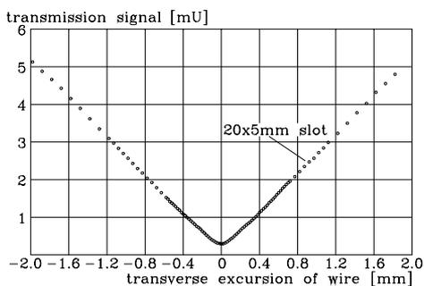
Figure 4: Measured transmission coefficient versus the wire shift for one slot length for prototype B.
