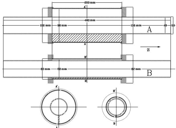
Figure 2: Longitudinal and transverse cut of the two prototypes.
