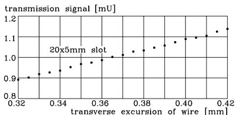
Figure 6: Measured transmission coefficient versus the wire shift for one slot length for prototype B.
