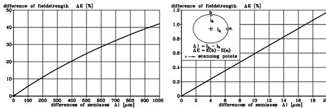
Figure 9: Relative difference of the field strength versus the ellipticity of the beam tube with a centered beam, taken at constant distance from the wall of the beam tube.
