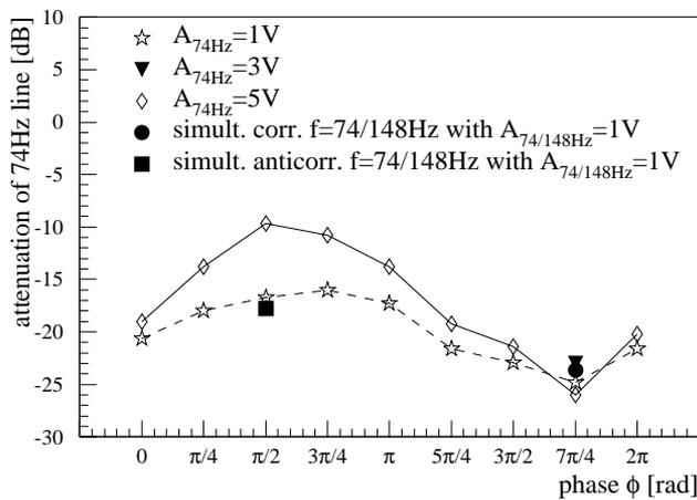
Figure 4: Harmonic compensation of the 74 Hz PS frequency and its first harmonic as function of the correction signal phase  $\phi$  and amplitude  $A$ .
