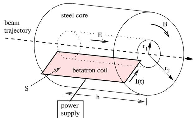
Figure 1: Schematic view of the betatron core.
