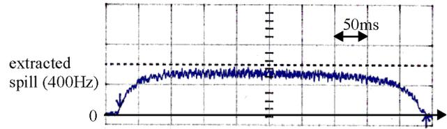
Figure 5: Extraction with servo system, BW 400 Hz.
