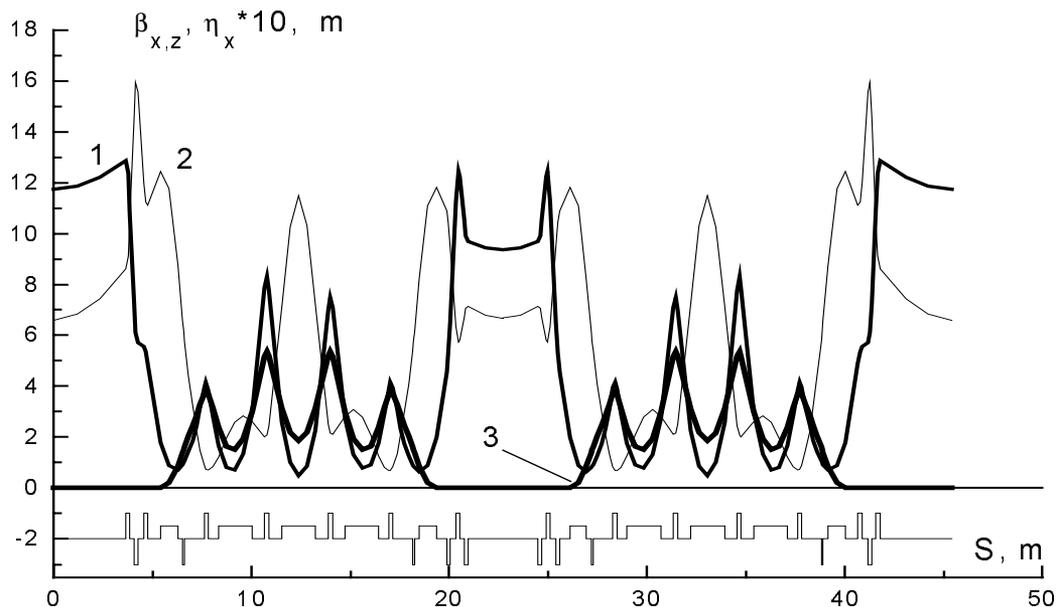
Fig. 2. Lattice functions  $\beta_x$  - (1),  $\beta_z$  - (2) and  $\eta_x \cdot 10$  - (3) the proposed ring in SLS operating mode.
