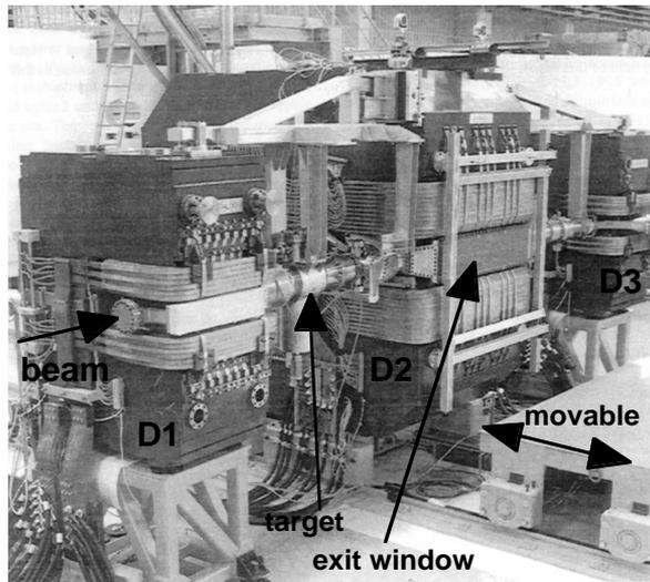
Figure 4: View of the ANKE facility. The reaction products penetrate the large exit window in the gap of D2 and are analyzed by detectors on the right hand side of D2. The bending angle can be varied between zero and 10.6 degrees.
