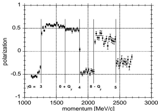
Figure 2: Polarization recorded during acceleration with the EDDA detector.
