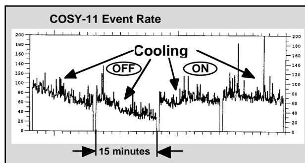
Figure 1: The COSY-11 event rate is constant over 15 minutes if the cooling system is on.
