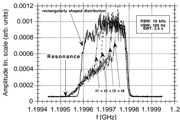
Figure 5: Stochastic extraction at 2.6 GeV/c. The noise is swept from the left over the shaped distribution.
