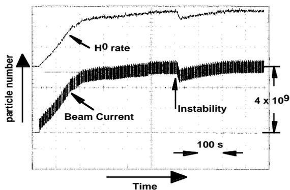
Figure 3: Stacking of protons with electron cooling. The beam is injected every 5 seconds. The stored intensity increases until an equilibrium is reached after about 180 seconds. As marked by the arrow an instability due to space charge prevents a further increase in intensity.
