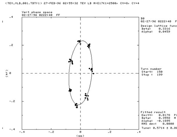
Figure 4. Fitted phase space coordinates in vertical plane.
