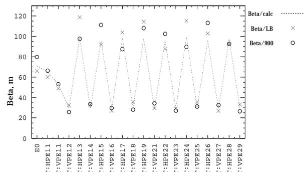
Figure 6. Section E1 & E2 horizontal beta plot of the low beta data, the 900 GeV data, and the design values.
