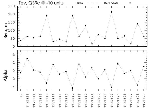
Figure 9. Lattice plot of data and calculation with harmonic quadrupoles giving a -10 unit cosine driving term.
