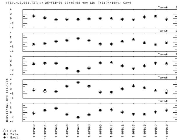
Figure 1. The horizontal BPM positions around the  $B\bar{O}$  collision point.
