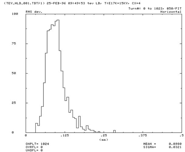
Figure 2. Histogram of horizontal BPM RMS deviation from the fitted positions.
