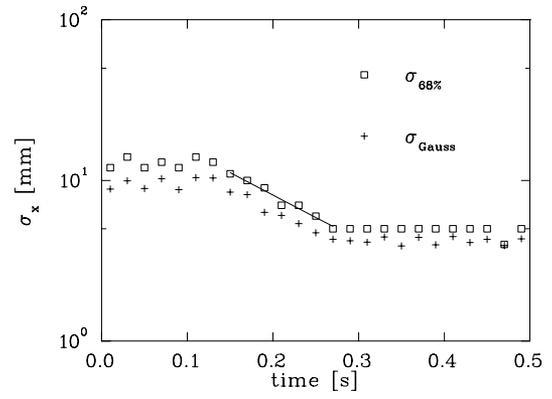
Figure 4: Measured horizontal beam width  $\sigma_x$  during electron cooling
