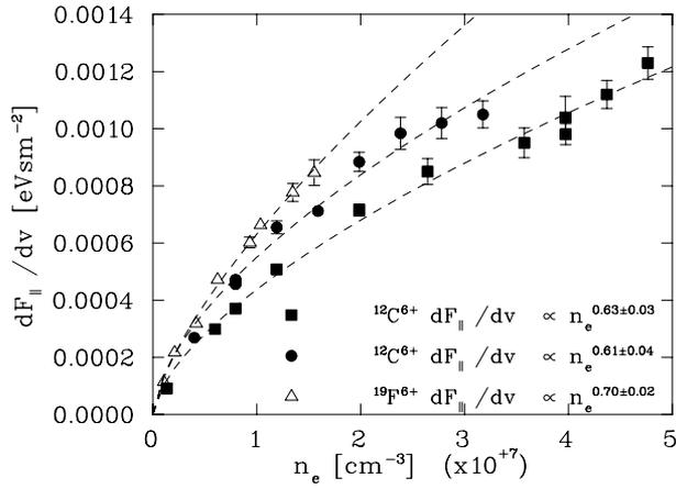
Figure 2: The slope of the longitudinal cooling force as a function of the electron density
