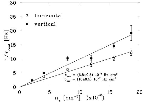
Figure 5: Measured horizontal and vertical cooling rates as a function of electron density
