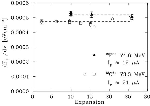
Figure 3: The slope of the longitudinal cooling force as a function of the expansion factor
