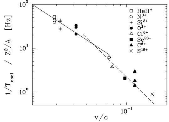
Figure 7: Normalized inverse cooling time as a function of ion velocity. The inverse cooling times are normalized to  $Z^2/A$  and an electron density  $n_e = 10^8 \text{cm}^{-3}$
