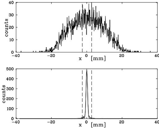
Figure 6: Measured beam profile in the horizontal plane for  $^{12}\text{C}^{6+}$  ions after multi-turn injection (top) and after 2 seconds of electron cooling (bottom).
