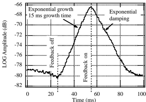
Figure 6: Typical growth/damping rate measurement (lower vertical sideband of  $1f_0$ ,  $I_{AV} = 80$  mA).
