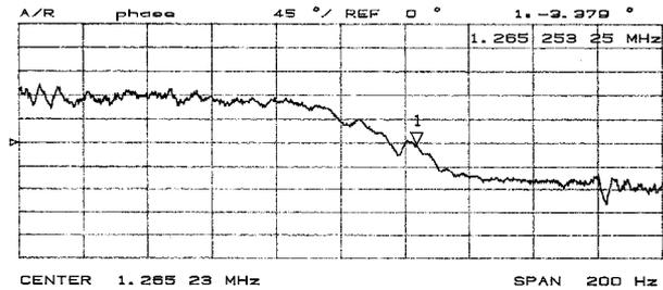
Figure 3: Lower horizontal sideband of  $873f_0$ .
