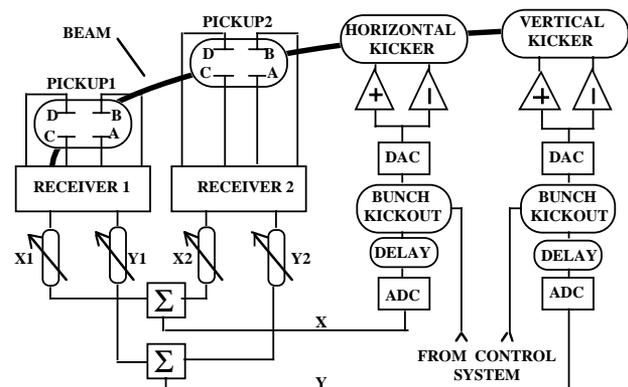
Figure 1: Transverse feedback system concept.
