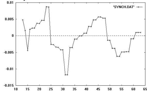
Figure 3. The relative deviations from linear increase,  $\Delta Br/(Br)$ , versus the magnet number of turn 2 to 5, showing two coherent synchrotron oscillations.
