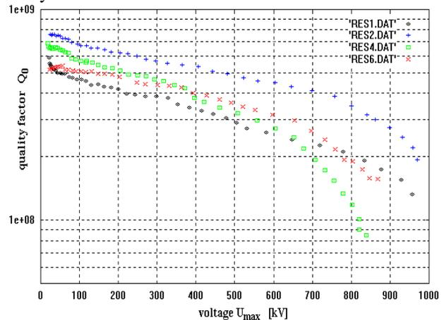
Figure 2. Typical curves of the unloaded quality factor of the Tritron cavities versus the voltage amplitude at the last beam hole.
