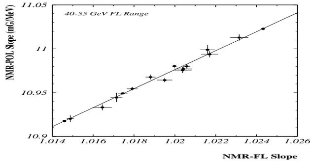
Figure 4: *NMR/Flux-loop* comparison in the calibrated energy range. Correlation between fitted slopes for *NMR* vs  $E_{\text{Pol}}$  and *NMR* vs  $B_{\text{FL}}$ . One point per *NMR* probe.
