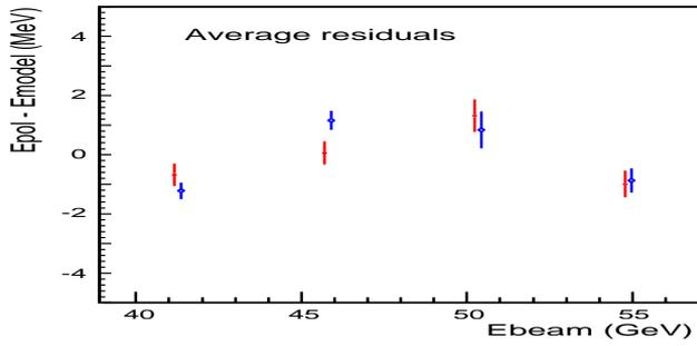
Figure 3: Non-linearity measurement in the *RD*-calibrated energy range. Residuals  $E_{\text{Pol}} - E_{\text{NMR}}^i$  averaged over all *NMRs* for the two fills with four calibrations. Error bars are rms of residuals for each set of *NMR* measurement.
