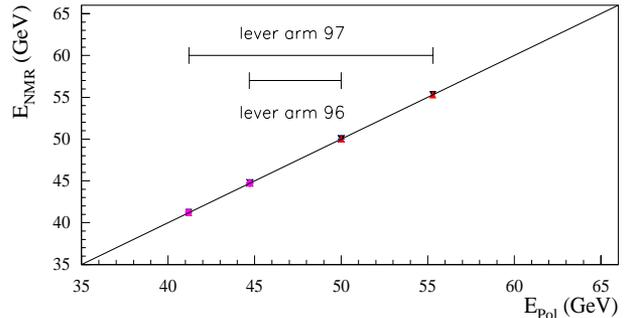
Figure 2: The improved range of calibrated energies.  $E_{\text{NMR}}$  represents the equivalent beam energy from *NMR* informations on the *B*-field in some of the LEP dipoles.
