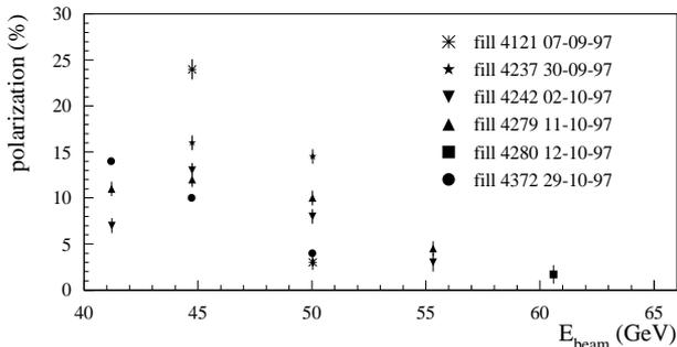
Figure 1: Polarisation measurements performed at four beam energies in different fills. Four energies were calibrated in the same fill on two occasions.
