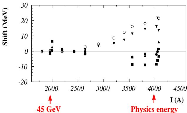
Figure 5: Example of extrapolation using *NMR/FL* correlation established in the *RD*-calibrated energy region.
