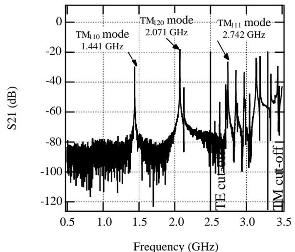
Figure 2:  $S_{21}$  spectrum measured from the vertical coupling probe to a  $45^\circ$  probe.
