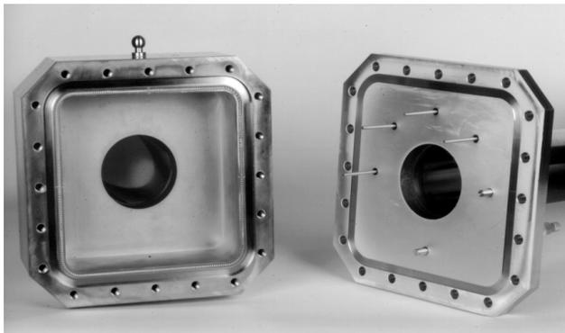
Figure 1: Cavity with cover plate removed to show rectangular cavity with (oversized) coupling probes, and tuners.
