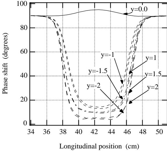
Figure 3: Phase shift due to perturbation of the  $TM_{120}$  mode by a needle at various  $y$  (vertical) offsets.
