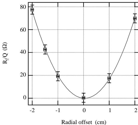
Figure 4: Measured  $(R_{\parallel}/Q)$  as a function of horizontal offset of the perturbing needle, with quadratic fit. No transit time correction has been applied.
