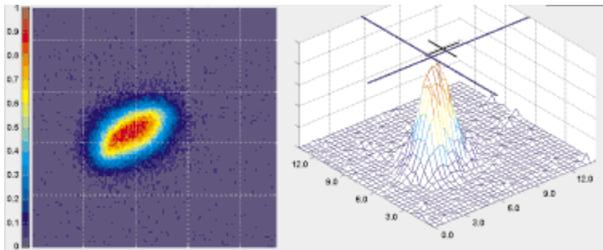
Figure 2: Beam profile for LEA experiment.
