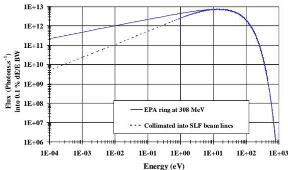
Figure 4: Photon flux in SLF lines (308 MeV, 115 mA).
