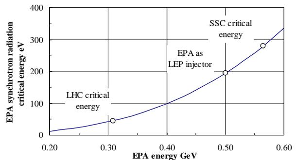
Figure 3: Critical photon energies versus EPA beam energies.
