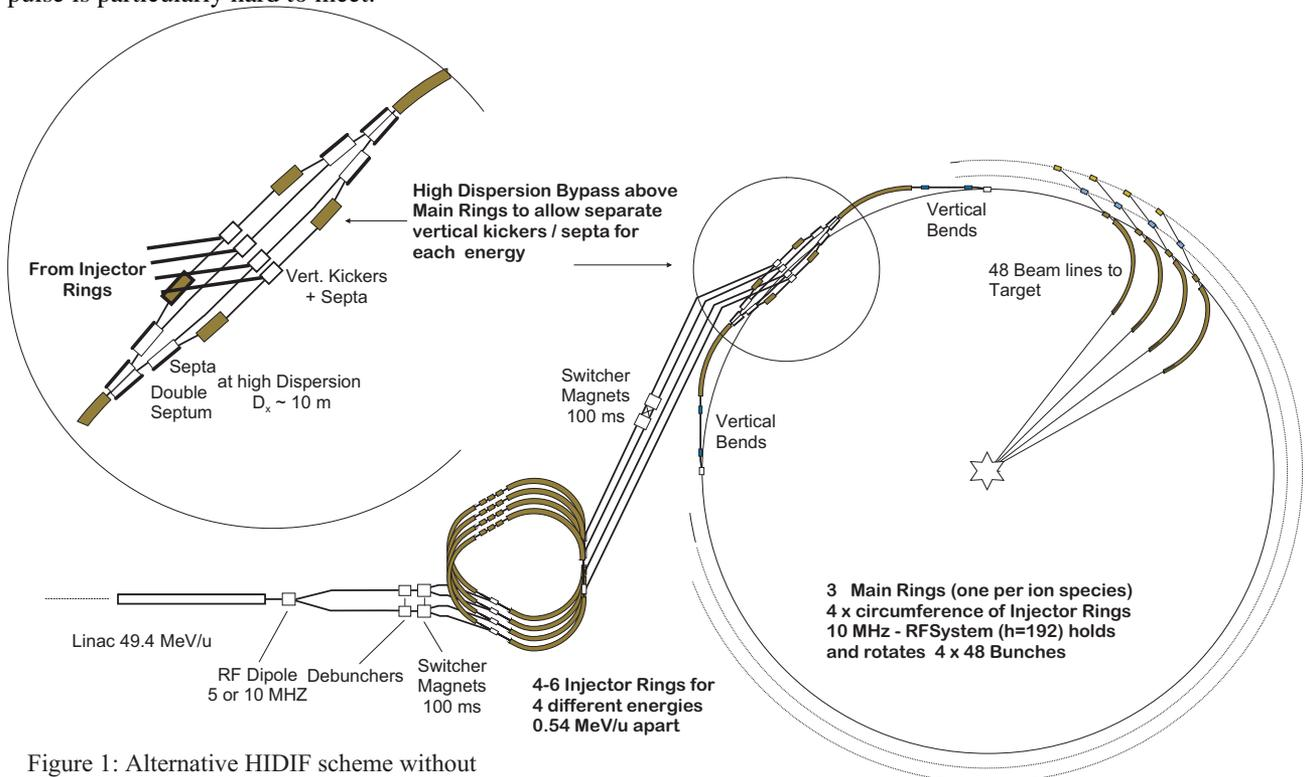
Figure 1: Alternative HIDIF scheme without external buncher induction linac
