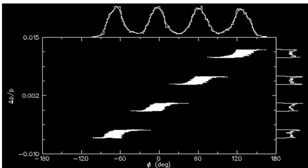
Figure 4: Rotated and aligned sub-bunches before extraction from the main ring.
