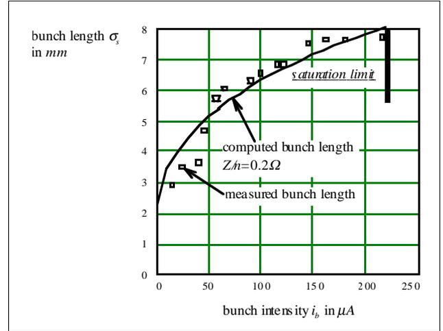
Figure 6 : Computed and measured bunch length at 22 GeV/c.
