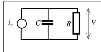
Figure 2 : Equivalent diagram of button electrode.
