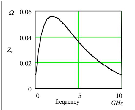
Figure 3 : Transfer impedance of button electrode and transmission cable.
