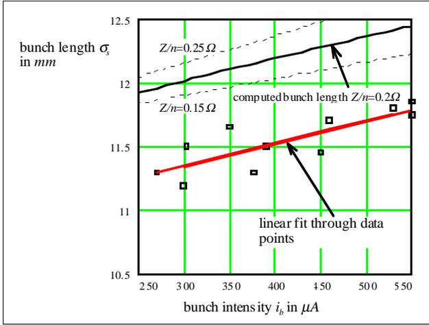
Figure 5: Bunch length as a function of single bunch intensity at 91.5 GeV/c compared with expected values when  $\text{Imag}(Z/n)=0.2 \Omega$ .
