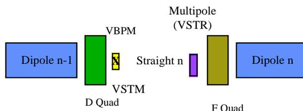
Figure 1: Schematic showing position of vertical correctors and monitors in an SRS lattice cell.
