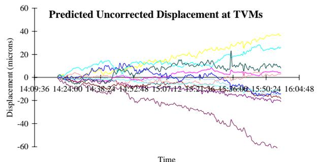
Figure 4: Predicted drift at TVMs without feedback
