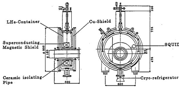
Figure 1: Design of the cryostat for the cryogenic current measuring device.
