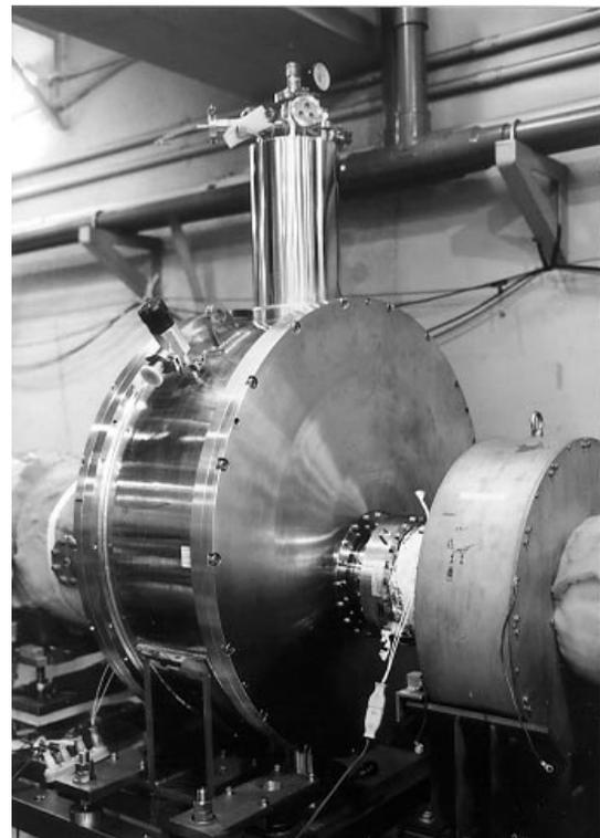
Figure 2: Photograph of the cryogenic current measuring device installed at the TARN II ring.
