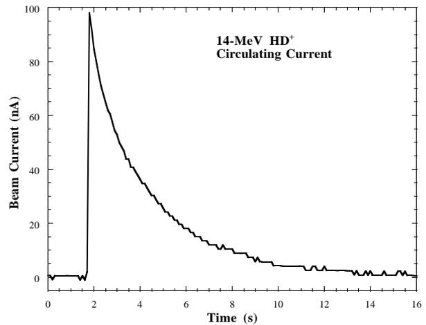
Figure 5: Measured ion current stored in the TARN II. The current decreases due to the dissociation of the molecular ion  $\text{HD}^+$ .
