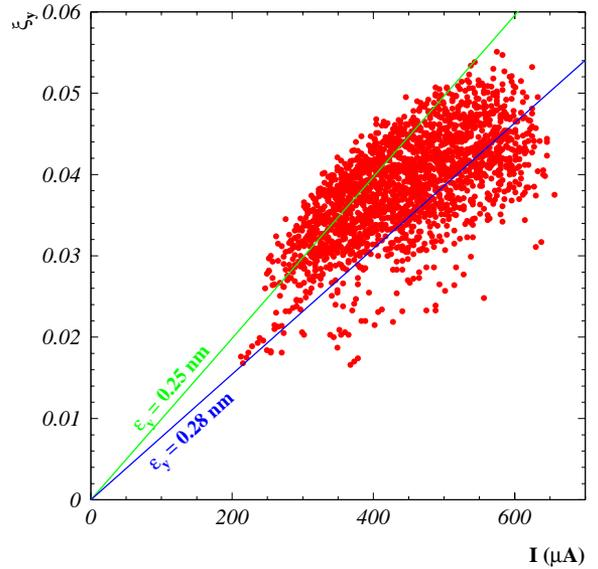
Figure 3: Vertical beam-beam tune shift  $\xi_y$  as a function of the bunch current ( $\beta_x^* = 1.5$  m). There is no strong evidence for a beam-beam limit. The lines show the expected dependences for two vertical emittances  $\varepsilon_y$ .
