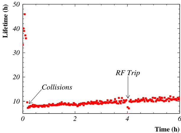
Figure 4: Evolution of the beam lifetime during a physics fill at 91.5 GeV. The initial lifetime is  $\sim 40$  hours. The sudden drop below 10 hours occurs when the beams are brought into collision. The lifetime increases with time as the bunch currents and the beam-beam tune shifts go down.
