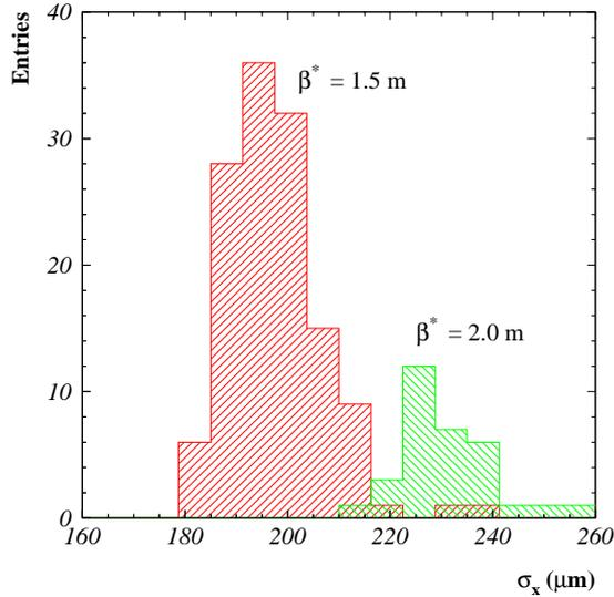
Figure 2: Horizontal beam sizes  $\sigma_x$  measured with beam-beam deflections scans for  $\beta_x^* = 1.5$  and  $2.0$  m ( $J_x = 1.6$ ). The mean ratio is 1.15 as expected from the  $\beta_x^*$  ratio.
