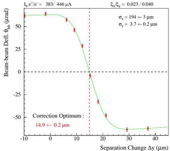
Figure 5: Example of a beam-beam deflection scan used to optimise the setting of the vertical separators. The beam sizes at the collision point  $\sigma_x$  and  $\sigma_y$  as well as the beam-beam tune shifts  $\xi_x$  and  $\xi_y$  are extracted from the fit to the data (line).
