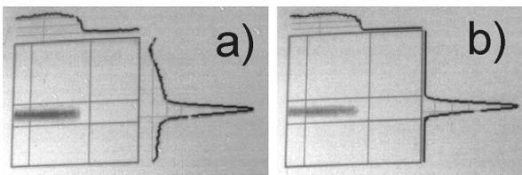
Fig.1 Image of SR beam cross-section and corresponding profiles a) before background discrimination, b) after background discrimination.
