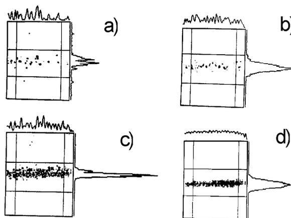
Fig.2 Image of SR beam and profiles on one TV frame for different storage ring beam current. a)  $I = 2.5 \text{ mA}$ , b)  $I = 5 \text{ mA}$ , c)  $I = 10 \text{ mA}$ , d)  $I = 25 \text{ mA}$
