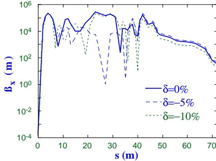
Figure 2: Final-focus beta functions for 10% different beam energies; on the right are linac-like FODO cells with  $\beta \approx 20$  m, on the left the IP with  $\beta = 150 \mu\text{m}$ .
