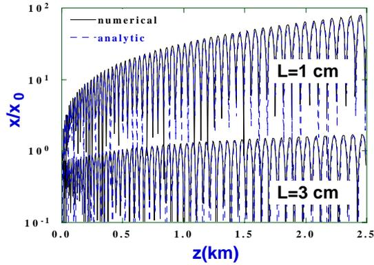
Figure 4: Simulated and analytical beam break up in the linac, without BNS damping.
