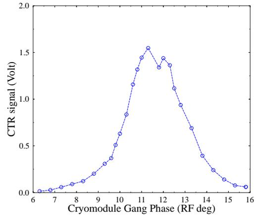
Figure 6: Coherent transition radiation signal measured by Golay cell vs. linac phase
