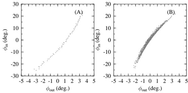
Figure 5: Comparison of measured  $M_{55}$  transfer map with the PARMELA calculated result for the second longitudinal pickup cavity.
