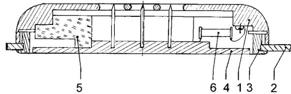
Figure 1: Schematic view of the flat corona triode. 1 - grid; 2 - intershield; 3 - flange; 4 - disk with points; 5 - isolator; 6 - leak resistor.
