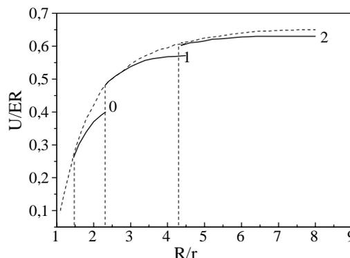
Figure 2: Dependence of voltage  $U/ER$  of electrostatic generator with optimum disposition of the intershields on the ratio  $R/r$ . 0 - without any shields; 1 - with one shield; 2 - with two intershields. The broken line shows the range where a corona from tank occurs.
