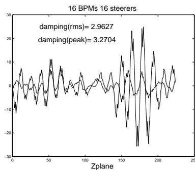
Figure 2: Example of static orbit correction obtained with our 16 BPMs/16 steerers system
