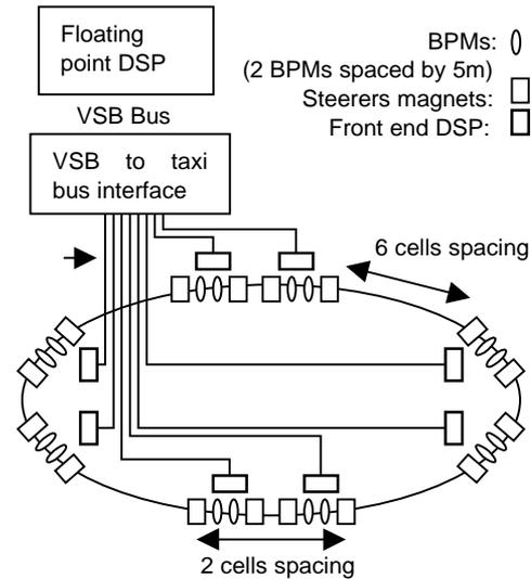
Figure 1: Layout of the global feedback system.
