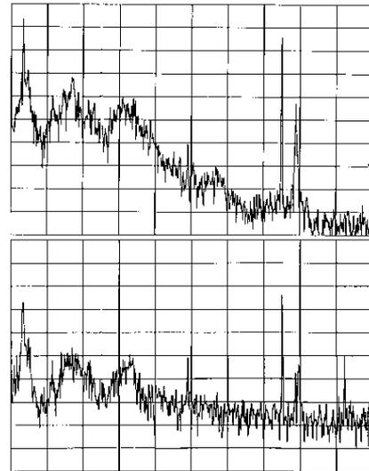
Figure 6 : Spectrum of an undulator X ray beam position 25 m away from the source with feedback off and on ( 5dB/div, 200 Hz span).
