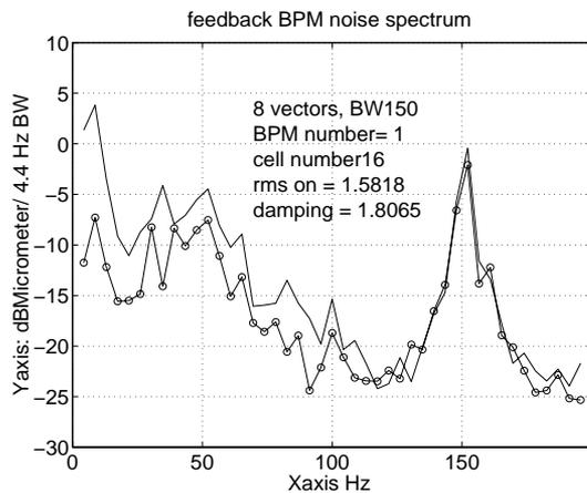
Figure 4: Spectrum of the beam position motion signal of a feedback BPM with feedback off and on
