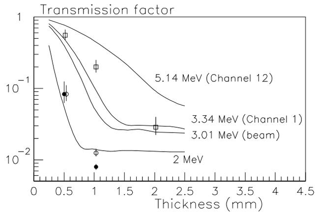
Figure 2: Transmission factors with stainless steel filters as a function of their thickness; channel 1 :  $\square$  (laser shots); channel 12 :  $\circ$  (laser shots),  $\bullet$  (gas BG noise runs). The error bars indicate the dispersion on several shots or runs. Continuous lines : simulation with EGS4.
