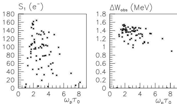
Figure 3: Variations of  $S_1$  (left) and of  $\Delta W_{obs}$  (right) with  $\omega_p \tau_0$ . The fitting procedure ( $S_1 > 10e^-$ ) introduces a cut off at  $\Delta W_{obs} = 0.85$  MeV.
