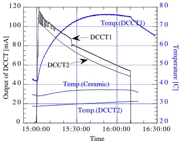
Figure 4 Another record of the single-bunch operation. The output of the DCCT1 fluctuated discontinuously at the high current.
