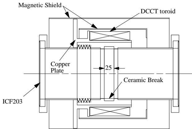
Figure 2 : Schematic view of the previously-installed DCCT duct.
