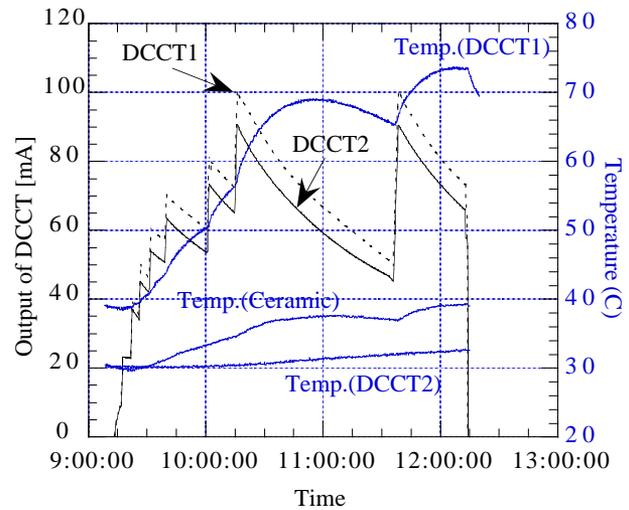
Figure 3 : A record of DCCT outputs and temperature at the single-bunch operation. No significant heating-up was observed for the newly installed DCCT2, in contrast with the previously installed DCCT1.
