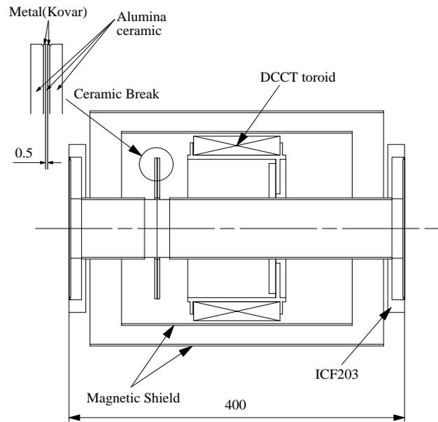
Figure 1 : A newly-installed vacuum duct for the DCCT. The ceramic break constitutes a capacitor of 2.6 nF.
