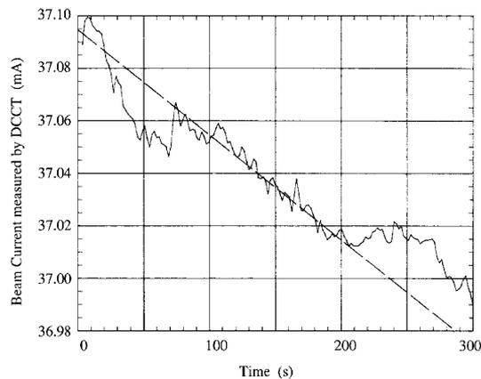
Figure 5 : Slow fluctuation observed in the output of the DCCT1 at the single-bunch operation.
