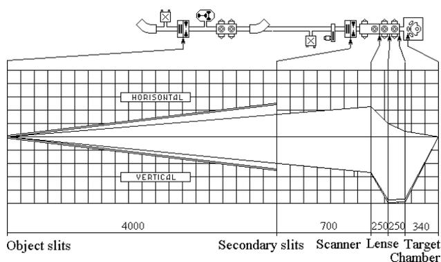
Fig.5 The layout of a microbeam facility. Sizes are given in millimeters.
