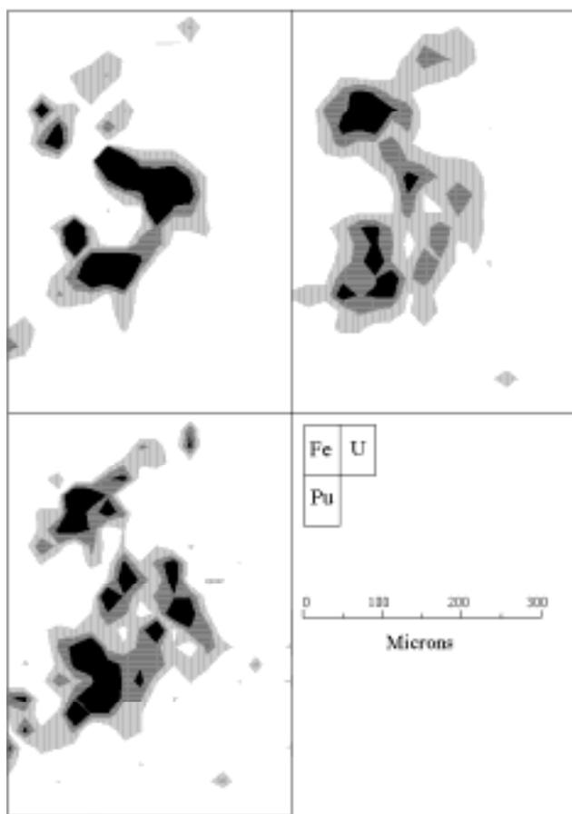
Fig.6 Maps of Fe, U and Pu distribution in the particulate from SNTS.
