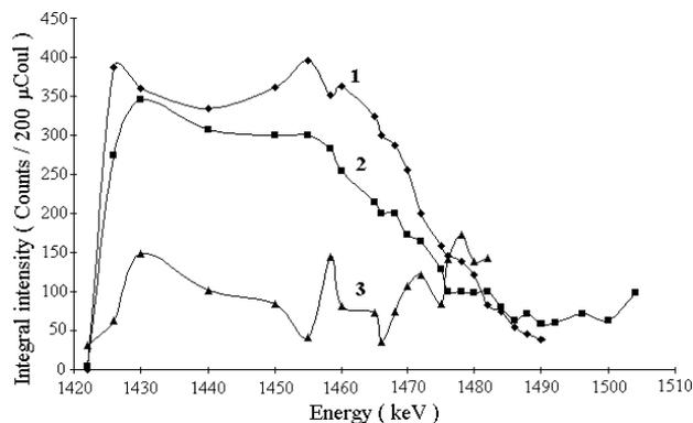
Fig.4 Characteristic NRA spectra for determination of Ni distribution before and after annealing
