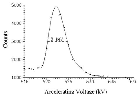
Fig. 1 Yield curve of nuclear reaction  ${}^9\text{Be}(p,\gamma){}^{10}\text{B}$ , energy of resonance 1084 keV
