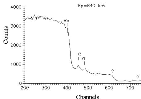
Fig. 3 Characteristic RBS spectrum resulting from irradiation of Be foil by protons with energy 840 keV.
