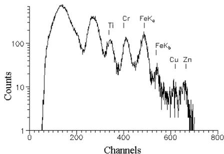
Fig.2 Characteristic PIXE spectrum resulting from irradiation of Be foil by protons with energy 680 keV.
