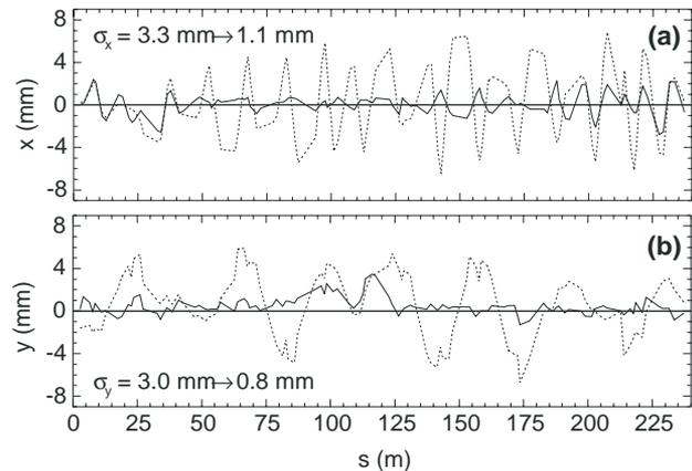
**Figure 6.** First results of horizontal (a) and vertical (b) orbit correction in the storage ring.
