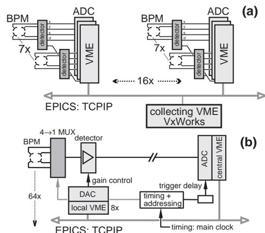
**Figure 4.** Overview of the SR BPM setup for closed orbit mode (a) and for single-turn (b).
