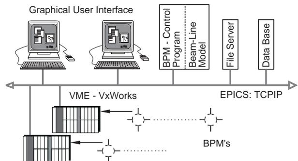
**Figure 2.** Overview of the signal processing. Pickup-signals are recorded and processed on VME-crates and made available on the network. Unix software tools are used for logging and orbit-manipulation.
