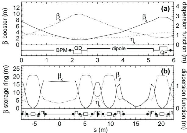
**Figure 1.** Machine functions in 1 of the 16 section of the booster (a) and in 1 of the 8 sections in the SR (b). Optical components and BPM-positions (dots) are indicated.
