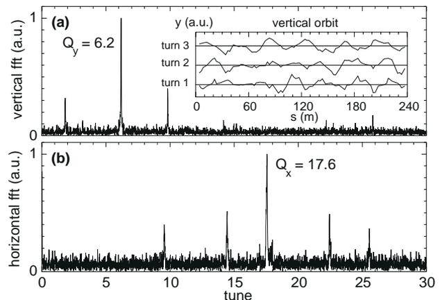
**Figure 7.** Tune-measurement obtained from 64 individual single-turn recordings (e.g., see inset).
