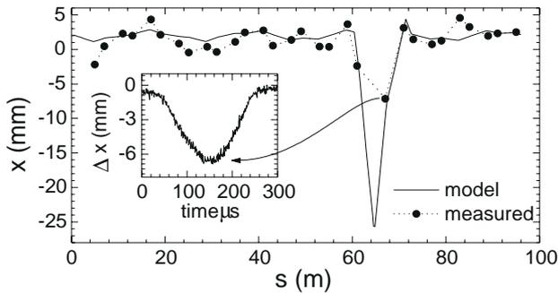
**Figure 5:** Measurement of the extraction bump of the booster compared with the optics model Goemon [6]. The inset shows the evolution of the marked BPM while the bumpers are fired.
