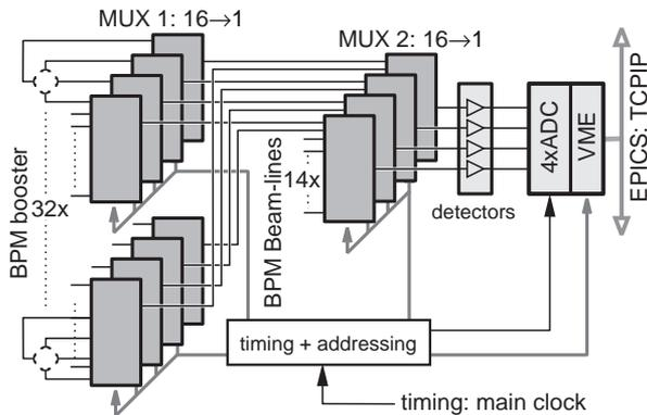
**Figure 3.** Overview of the injector BPM setup.
