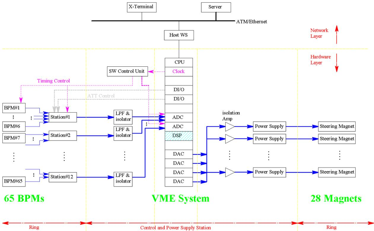
Figure 1: Block diagram of the global feedback system. Station#1-#12 contain multiplexers and superheterodyne detectors. (LPF:Low Pass Filter, ATT: Attenuator, SW Control: Switch control)
