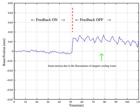
Figure 4: Beam motion at BPM#50.
