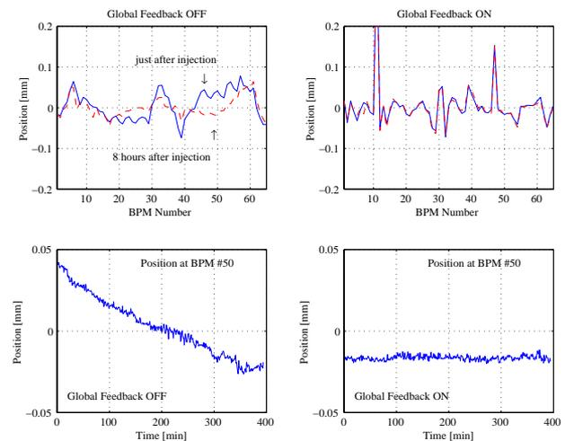
Figure 2: Change in COD without feedback (upper left) and with feedback (upper right) in eight hours. The peaks at the BPM#11 and #47 are due to the trouble of the electrodes. Lower left and right graph show the position change at BPM#50.
