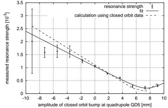
Figure 3: Harmonic correction of the imperfection resonance at 1.32 GeV using a closed orbit bump.
