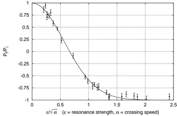
Figure 2: Change in polarization level due to crossing of the imperfection resonance at 1.32 GeV.
