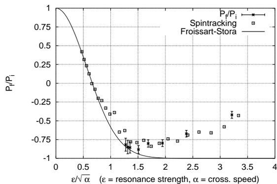
Figure 4: Change in polarization level due to crossing of the imperfection resonance at 1.76 GeV.
