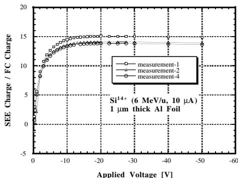
Fig. 4 : Time-varying Plateau curves for the 200  $\mu\text{A}$  peak  $\text{Si}^{14+}$  beams.
