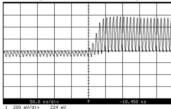
Fig. 6 : A fast timing signal observed from the SEEM for the 10  $\mu\text{A}$  peak  $\text{C}^{6+}$  beams. Data is given by 200 mV/div and 50 ns/div. The pulse height of the induction of the beam passage is about 130 mV.
