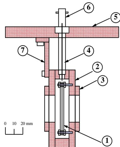
Fig. 1. A cross sectional view of the SEEM being used at the HIMAC injector(6 MeV/amu): 1 Three 1  $\mu\text{m}$ -thick Al foils, 2 and 3 Field adjusting flange, 4 Cu pipes, 5 130 mm $\phi$  vacuum flange, 6 SMA connectors, 7 Supporting plate.
