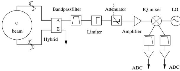
Figure 2: Signal processing scheme for TTFL cavity BPMs; only the y-channel is shown
