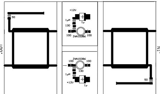
Figure 4: RF-amplifier - board layout and parts
