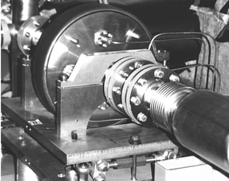
Figure 1: Warm monitor installed in the TTFL
