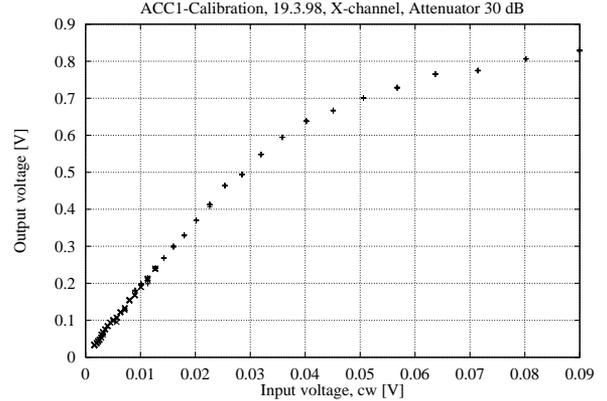
Figure 5: Linearity of the electronics measured after the calibration. The 30 dB-attenuator was switched ON.
