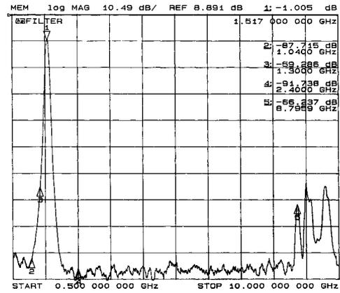
Figure 3: Bandpass filter with a center frequency of 1.517 GHz, measured insertion loss and stopband rejection
