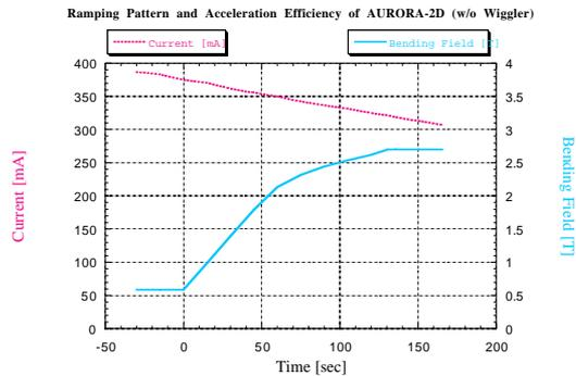
Figure 5: Typical acceleration pattern of A2D.
