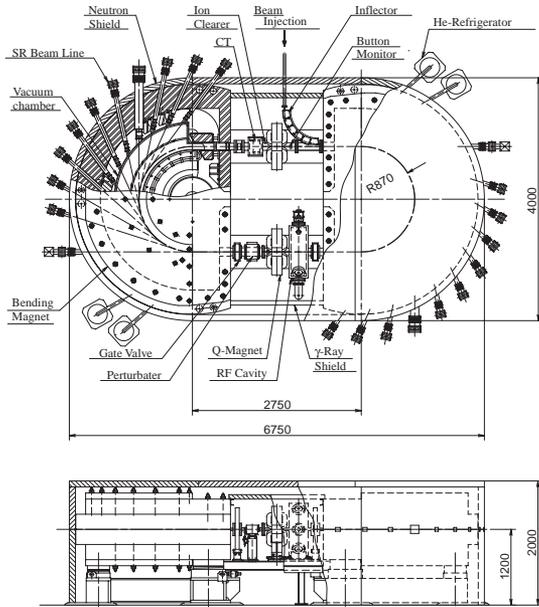
Figure 2: Schematic of A2S.
