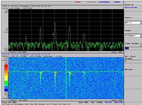
Figure 6: Damping time measurement at injection.
