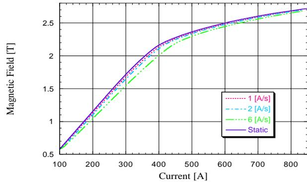
Figure 4: Dynamic excitation characteristics of 2.7 Tesla bending magnets.
