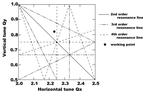
maximum value of the dispersion is 3.7 m at QFX. A tune diagram of the ring is shown in Fig. 3.
