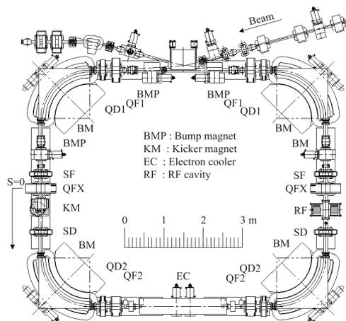
the QF2 and QD2. One of the criterion on designing the quadrupole magnet is that the magnetic field strength should be 0.75 T or less on pole tips.
