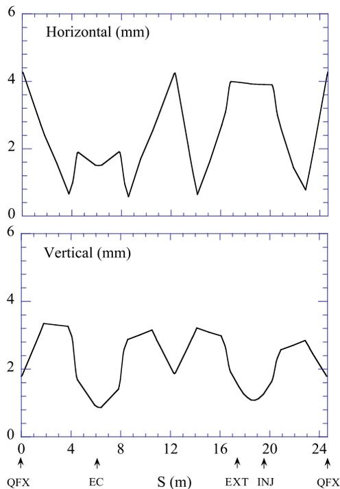
Fig. 4 : A standard deviation of COD along the beam axis estimated with 100 examples. A distance parameter  $s$  is measured from the center of the QFX.
