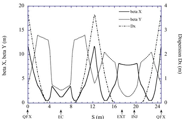
Fig. 2: Lattice functions of the small ring. A distance parameter  $s$  is measured from the center of the QFX. A solid line shows  $\beta_x$ , a dashed line shows  $\beta_y$ , and a dot-dashed line is a horizontal dispersion function  $D_x$ . EC, EXT, and INJ are the positions of EC solenoid, extraction, and injection respectively.
