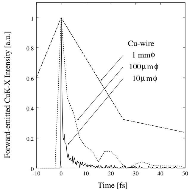
Figure 3: CuK-X pulse shapes for various sizes of copper wire.
