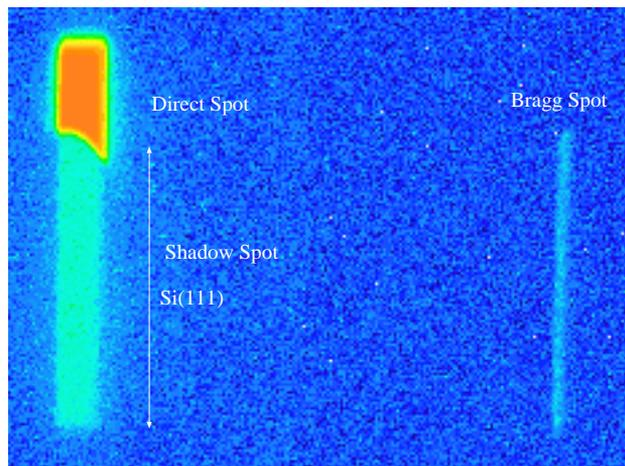
Figure 5: Si(111) diffraction image for 15  $\mu\text{m}^t$  copper foil.
