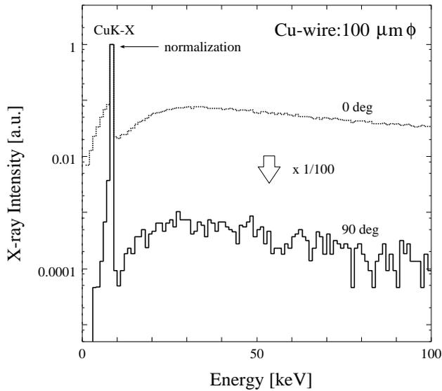
Figure 2: Comparison of (a) forward-emitted and (b) side-emitted X-ray spectra.
