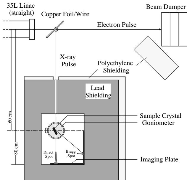
Figure 4: Experimental setup of the X-ray diffractometry at NERL linac.
