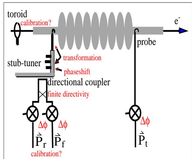
Figure 1: The signals for System Identification
