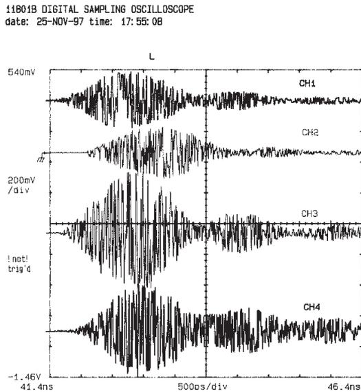
Figure 4: Signal voltages (peak to peak) measured after 15 m long cables and a bandpass filter for all channels, from top to bottom: CH1 364 mV, CH2 334 mV, CH3 804 mV, and CH4 588 mV.
