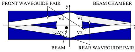
Figure 3: Profile of the beam chamber with four waveguides building up one BPM.
