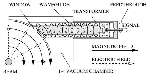
Figure 2: Sketch of the coupling mechanism.
