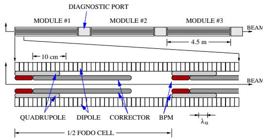
Figure 1: Sideview of the FEL-undulator (top) and zoom into focusing structure (bottom).
