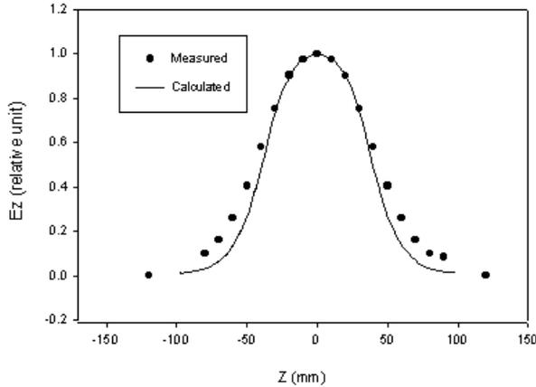
Figure 5: Electric field profile on the axis for the fundamental mode of the kicker.
