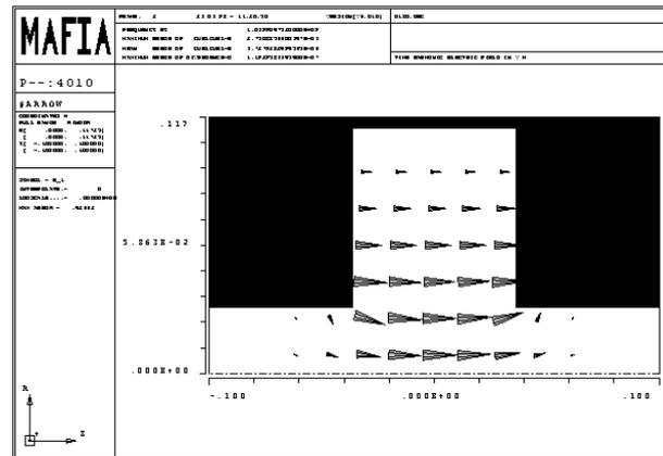
Figure 1: Electric field distribution for the E010 cavity.
