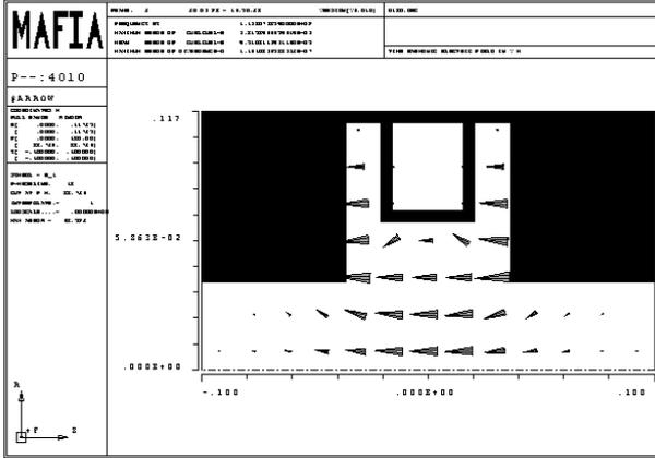
Figure 2: Electric field distribution for the fundamental mode of the kicker. The matching loads in the calculation are replaced with short circuits for simplicity.
