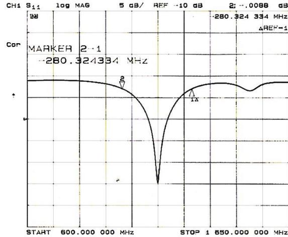
Figure 4: Reflection signal from the kicker, measured by network analyzer.
