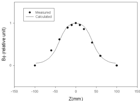
Figure 6: Magnetic field profile on the axis for the high order mode of 1492 MHz.
