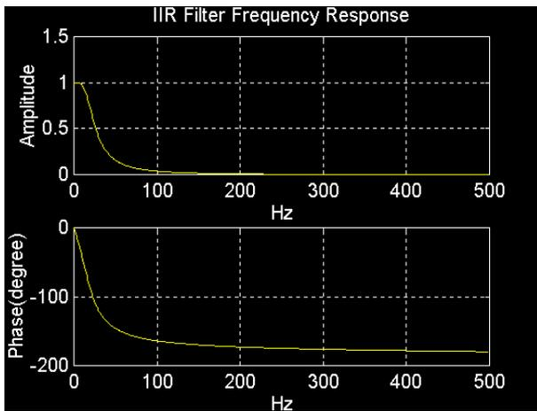
Figure 2: Frequency response of IIR filter.
