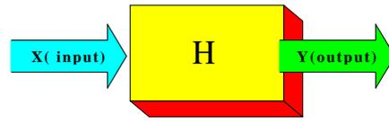
$$H(z) = \frac{B(z)}{A(z)} = \frac{b(1)+b(2)z^{-1}+\dots+b(n+1)z^{-n}}{1+a(2)z^{-1}+\dots+a(n+1)z^{-n}} \quad (1)$$
