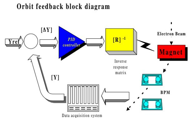
Figure 3: Local orbit feedback block diagram
