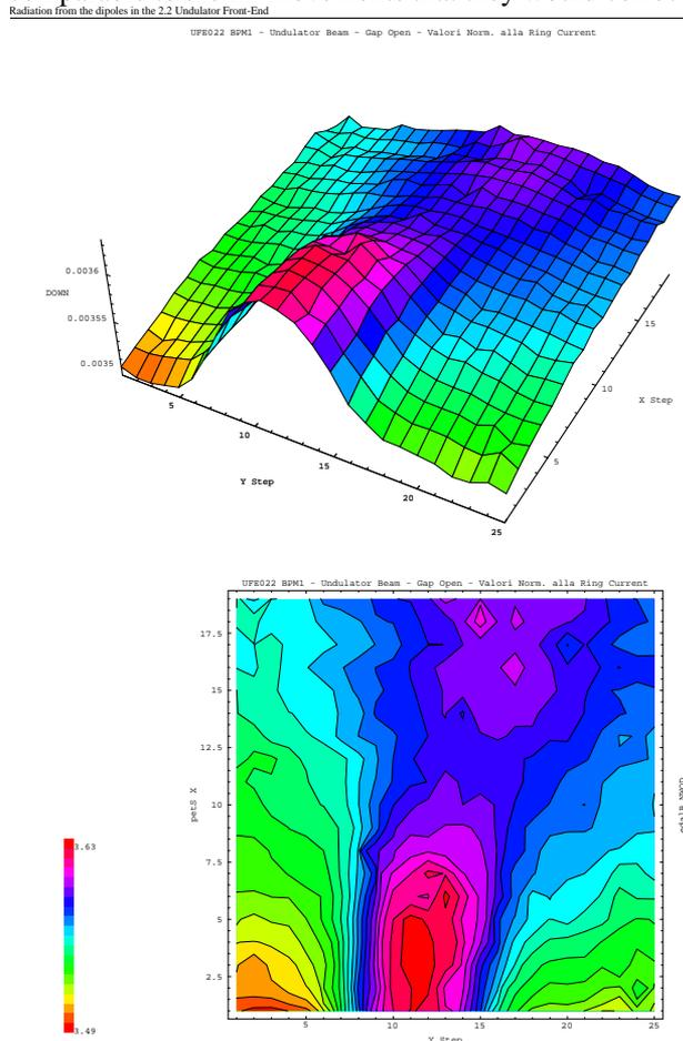
Figure 3: A real displacement of the dipole radiation detected in the undulator beamline from the section 2.2. There are clearly visible the two spots with different sizes and intensity.
