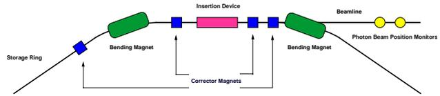
Figure 1: The layout of a straight section and the front-end of the beamline.
