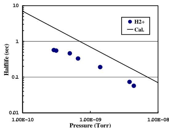
Fig.2. The dependence of the halflife of  $H_2^+$  on the vacuum pressure. Closed circles and solid line indicate measured and calculated halflife, respectively.
