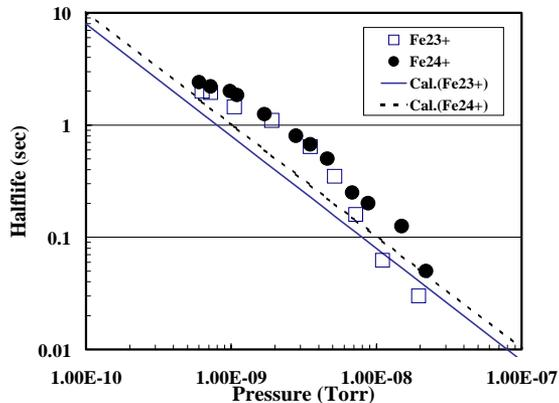
Fig.4. The dependence of the halflives of  $\text{Fe}^{23+}$  and  $\text{Fe}^{24+}$  on the vacuum pressure. Closed circles and open squares indicate measured halflives of  $\text{Fe}^{23+}$  and  $\text{Fe}^{24+}$ , respectively. Solid and broken lines indicate calculated ones of  $\text{Fe}^{23+}$  and  $\text{Fe}^{24+}$ , respectively.
