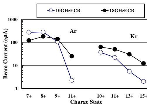
Fig. 1. Comparison between beam current of Ar and Kr from 18GHz-ECR and that from 10GHz-ECR.
