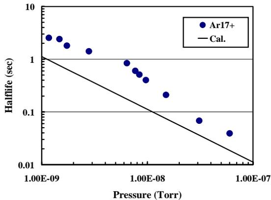
Fig.3. The dependence of the half-life of  $\text{Ar}^{17+}$  on the vacuum pressure. Closed circles indicate measured half-life and solid line is calculated one.
